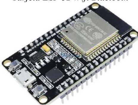
Figura 1 Tarjeta ESP 32 Wifi Bluetooth
